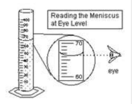
Meniscus – The concave surface of a liquid resulting from surface tension.
